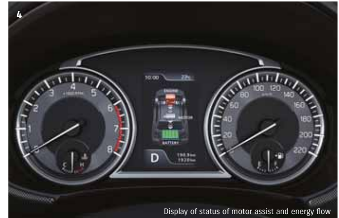
Display of status of motor assist and energy flow
